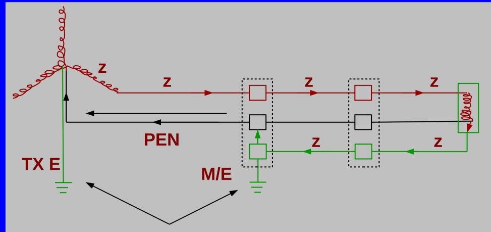
Barely any current runs through the ground as the impedance is much higher than the PEN conductor
